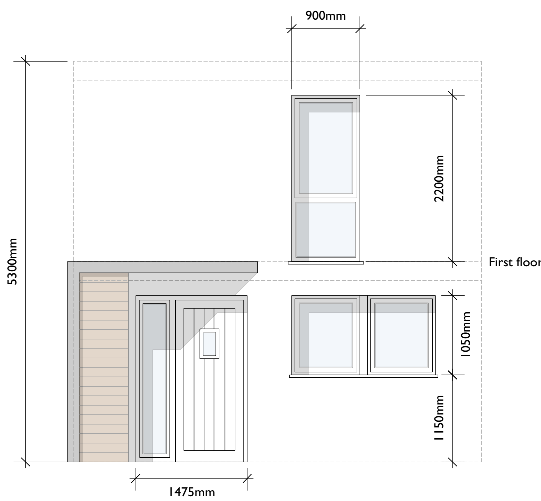
5 SIMPLE FRONT ELEVATION 320F Scale: 1:50
